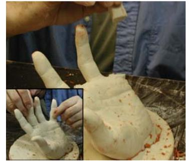
You can fix the cast straight out of the mold, using small steel tools to remove any bubbles or repair seam lines.
