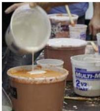
Pour a quarter of the mixed plaster into the mold and “skim coat” the mold by holding it and slowly rotating the mold - rolling the plaster around inside. This will coat the surface of the mold with a thin layer of plaster and deter bubbles from forming on the surface of your casting. When the inside seems completely coated (it may be difficult to see
