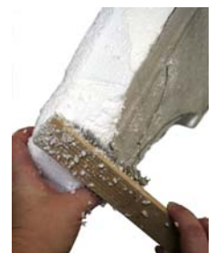
Image #5 Shaping with a wire brush
