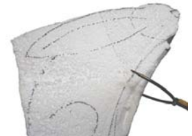
Image #4 Using Hot Wire Tool
